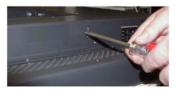
b) Remove the blank panel by pushing down slightly on the inserted end of the panel as you pull it out.
